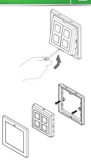
**4.** Replace the switch centre unit and clip the faceplate back into place. Make sure that the faceplate hooks in from the top as shown. A sharp click will indicate that the plate has been successfully replaced.
